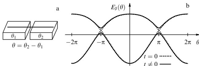
Figure 5. A Josephson junction made of quantum wire.
